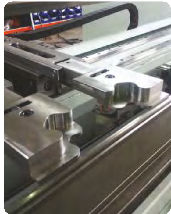
Special designed stop fingers for high accuracy and maximum flexibility even for conical bends
